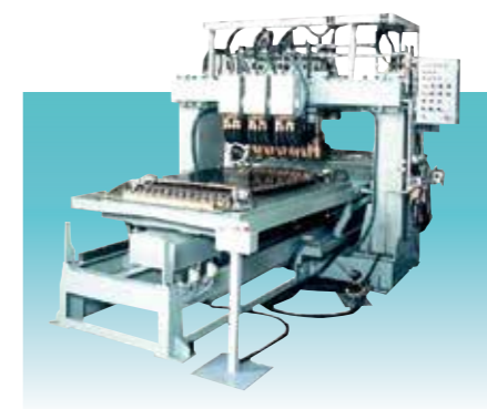
NC seam welders for six rows of solar collector panels
