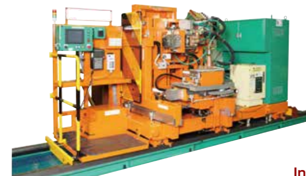
CNC inverter spot welders for underframes and side plates
